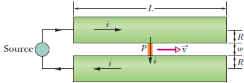
1. Show that the force on the projectile is directed to the right along the rails and is given approximately by
