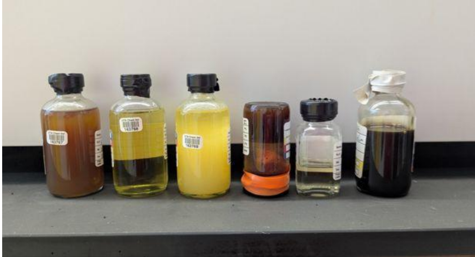
picture showing six different pyrolysis oils, each unique in color, clarity, and viscosity due to their unique chemical makeup
