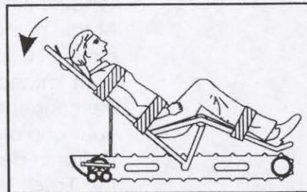
2. Then squeeze the Brake Release Bar with both hands. This will deploy the Front Auxiliary Wheels, making Evacu-Trac easier to push.
